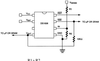
$$V_{\text{SENSE}} = \frac{R1 + R2}{R2} \times 1.25$$
